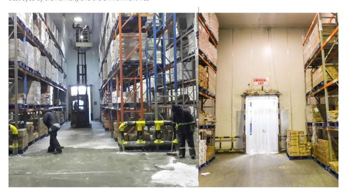
After SCE installed three DST dehumidifiers. There has been no ice formation, water pooling on the floor and the fog has been eliminated. Images borrowed by SCE.
